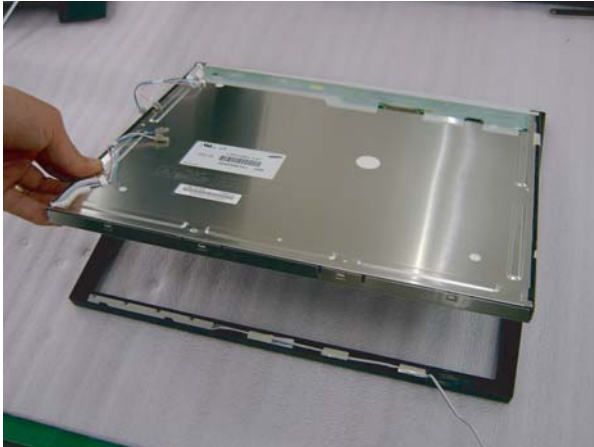
6. Lift up the LCD panel.
